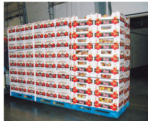
Unitized pallet loads are staged in the distribution center for shipment to the clubstores. Eliminating cornerboards saves the stores in time and labor.
