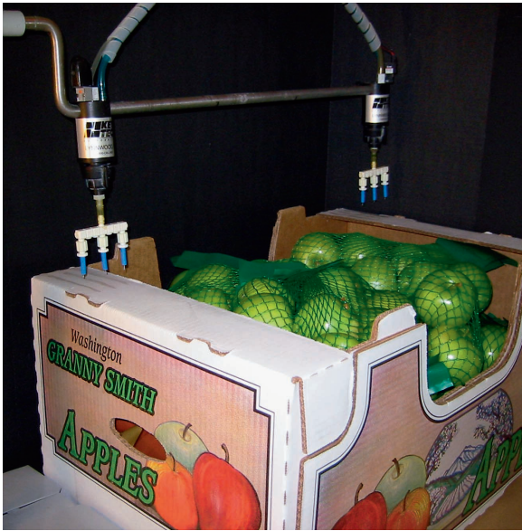
Easy-release adhesive is sprayed from nozzles onto the trays of produce as they convey to the palletizer in the Monroe Township, NJ, distribution center.
